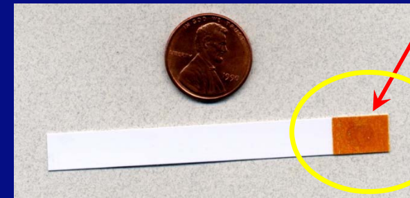
Flow-through (aperture) style reagent pad
