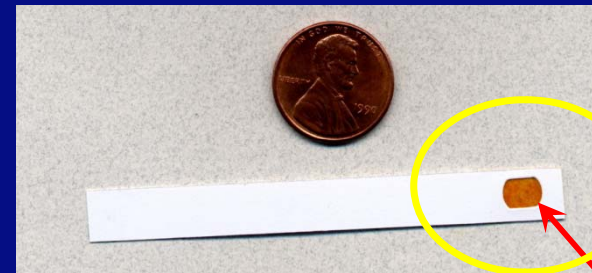
Flow-through (aperture) style reagent pad
