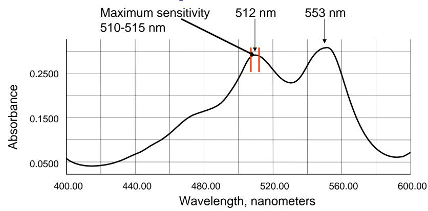
•Hach CI-17 on-line analyzer: 510 nm
